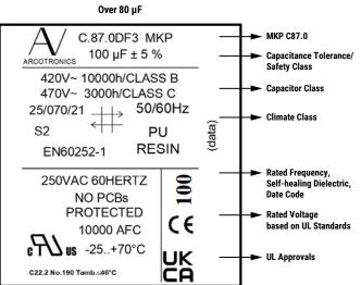
(data): Manufacturing Plant, Date Code, Day of Production, Internal Mark UL810: Applicable if inline with "Marking" from page 1
