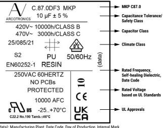
(data): Manufacturing Plant, Date Code, Day of Production, Internal Mark UL810: Applicable if inline with "Marking" from page 1 (data): Manufacturing Plant, Date Code, Day of Production, Internal Mari UL810: Applicable if inline with "Marking" from page 1
